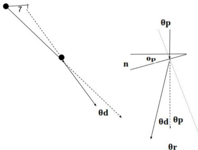
$$n \text{ sen} \theta_p = \text{sen} \theta_r \Rightarrow n \theta_p = \theta_r = \theta_d + \theta_p \Rightarrow \theta_d = (n - 1) \theta_p = \theta_p / 2$$
